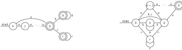
Fig. 4. A (k + 3) -state and a (k + 4) -state NFA accepting L_k and L_k^R of Theorem 13.
